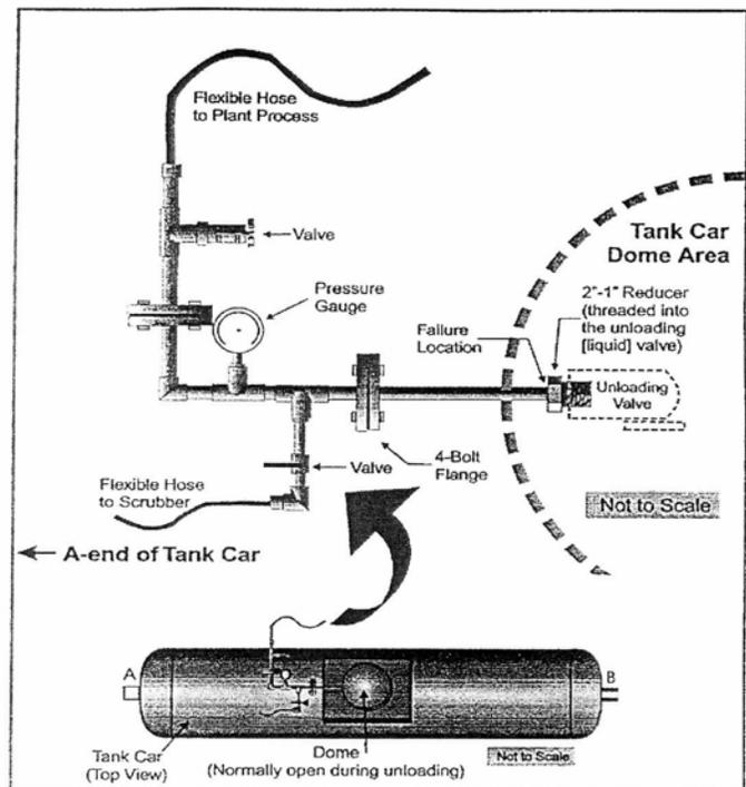
Overhead view of unloading apparatus. (For clarity, the pressure gauge, valves, and scrubber line have been rotated into the horizontal plane.)
