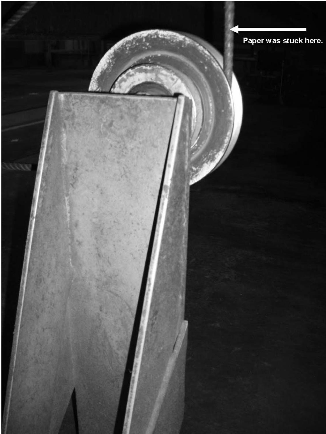
Fig. 7-1. Pulley where paper was stuck on rope.
