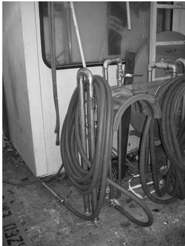
**Fig. 32-2. Air hose that was used to assist cutting dryer wrap.**
