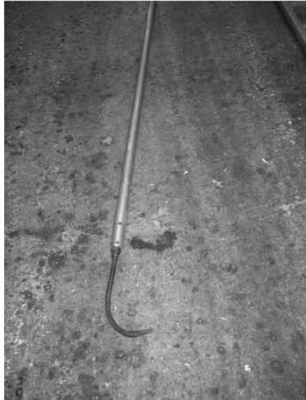
**Fig. 32-3. Long pole used to cut dryer wrap.**
