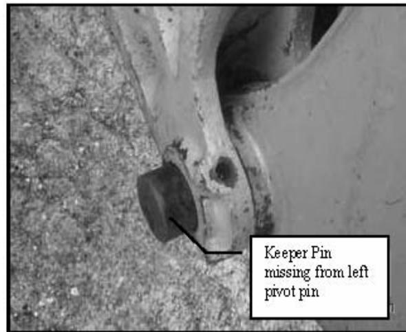
Operators had reported high vibration of the equipment's lower end. It was felt that this was due to inexperienced operators using the backhoe and lack of lubrication causing undue wear on the equipment. The vibration was most likely the cause of the keeper pin being missing.
